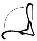
Fold the davits, etched parts 26 in half so that the relief etched detail is outermost. Fix the halves together with adhesive. Two sets of davits have been provided in this set for the boats on the port and starboard sides. These parts replace the kit parts 11 directly.
